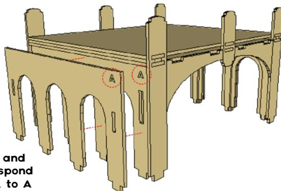
**IMPORTANT!** The "A" and "B" outer plates correspond to the inner plates (A to A and B to B). This is important to ensure you can clip to other I-48 pieces
