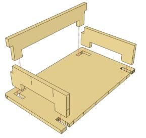
The pegs extend through the base piece to form lugs for locking into the building
