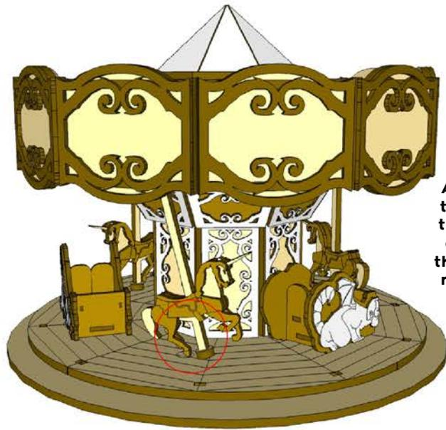
Apply glue to both the top and the bottom of the unicorns, and insert at an angle. Line up the base with the round mark on the base and straighten them up
