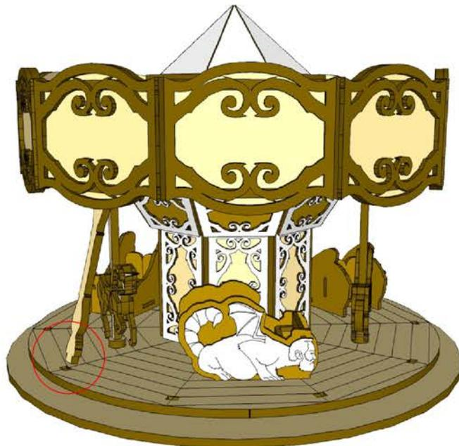
The posts go in at an angle and insert into the slots on the base. The top should glue to the top plate
