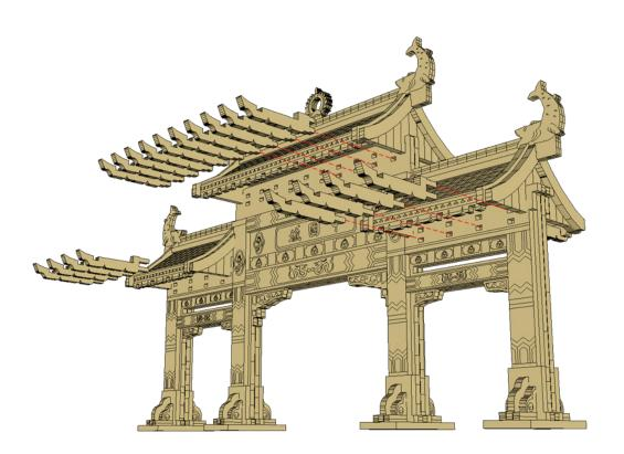
The struts have a slight upward sweep to them. To acheive this, insert the pegs into the main body of the gate, then push up to get them into the proper position
