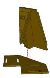
Glue the struts to the face plates and set aside to let it dry for a while. If you assemble several walls at once you can get a nice assembly line going, giving the first wall time to let the glue grab. This will make it easier to aseemble later.
