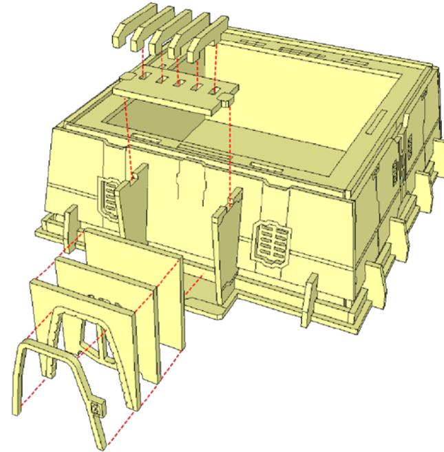
Glue the wall struts first and set aside to dry while you work on the next few steps
