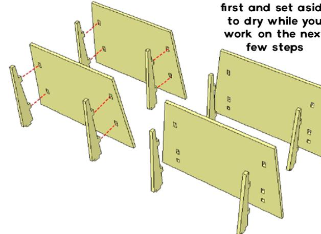
**Glue the wall struts first and set aside to dry while you work on the next few steps**
