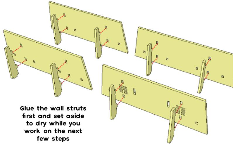
Glue the wall struts first and set aside to dry while you work on the next few steps
