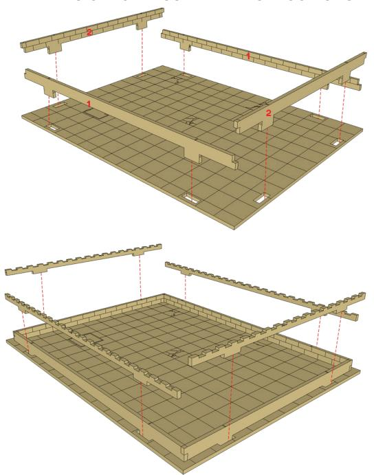
Glue the roof trim in the numbered order. The pegs extend through the roof piece to form lugs for locking into the second floor
