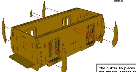
are placed lognest to shortest starting from the top. The middle fin pieces hasa longer tab that extends through the outter layer to plug into the layer below to help align the piece. The longest middle fin in located in the centre.a
