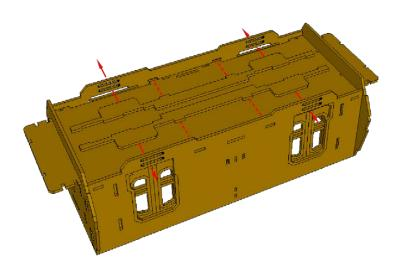
Be careful with you glue during this step. You want to make sure the glue doesn't squeeze out into the area where the round hole is. This hole is to allow the undercarriage pieces to 'swivel', so try to keep the area free from glue.
