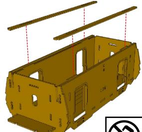
The doors are designed to slide open and closed. If you want this cool functionality on your model, don't use glue during this step and be careful when gluing in the runners underneath during the next step.
