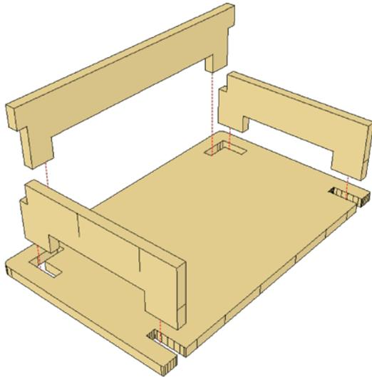
The pegs extend through the base piece to form lugs for locking into the building
