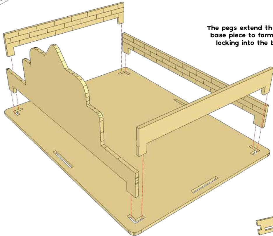
The pegs extend through the base piece to form lugs for locking into the building
