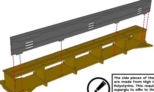
The side pieces of the tracks are made from High Impact Polystyrine. This requires superglu to affix to the MDF parts. Attaching these pieces can be deceptivly tricky, so take care qhwn applying your glue. You will need a bead of superglue running the length of the rail as well as the two end pieces and on the tabs at teh bottom
