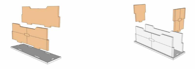
Install the long walls first, and then place the two shorter end piece sin place. We find it easier to use PVA on the bottom of the walls, and then once the shorter end pieces are in place run a bed of super glue on the inside.
