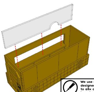
We use a non-fogging superglue designed for gluing clear parts to afix our acrylic pieces. The brand we use is Loctite Glass. It is worth hunting around in your local hardware store for a similar glue!
