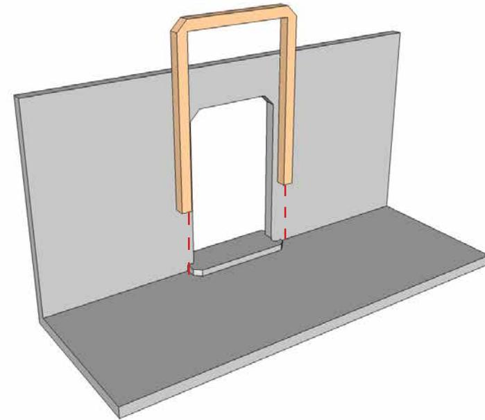
**The door frame goes on the inside of the model. The bottom legs of the frame should fit over and around the plate you just inserted. Try to make sure the frame is inserted straight and doesn't dry on an angle.**
