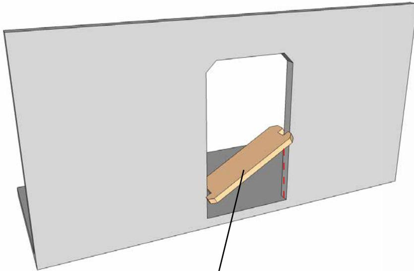
**This piece is designed to be inserted on an angle. Look for the square notches and place that inside the door opening on an angle and push it down into place.**
