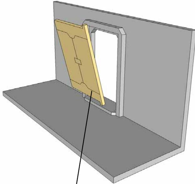
The best way to insert the door is to place the bottom peg in the hold in the bottom door plate and then rotate it up into position. It will sit loosely in place so you might need to hold it whilst you put the top plate in the next step in place.
