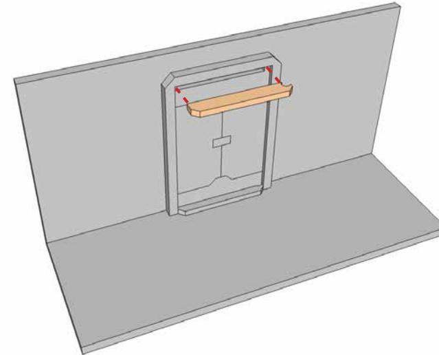
Once the door is in place you can slide the top plate in. It will slide in above the door and below the door frame. You might need to wiggle it a little so that the circular cutout slips over the small peg at the top of the door.
